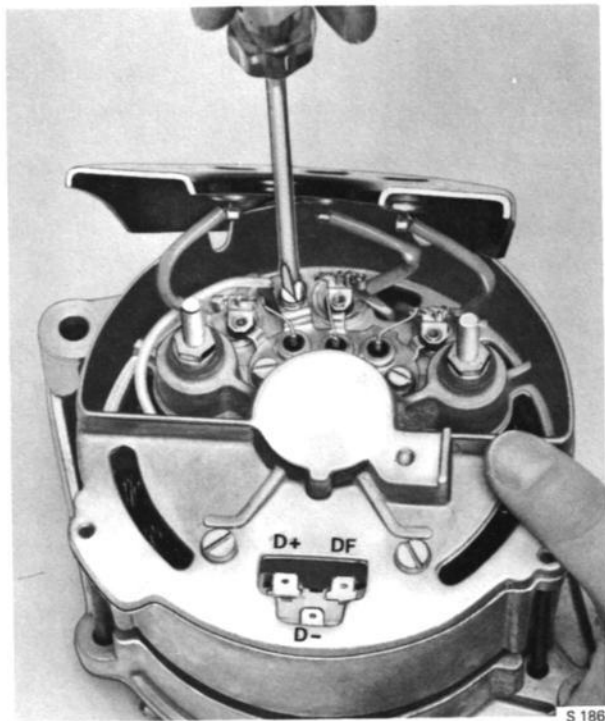
DISCONNECTING THE BRUSH UNIT ASSEMBLY WIRE
