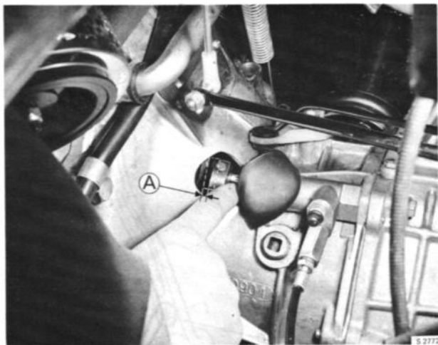
ADJUSTING THE CLUTCH CLEARANCE A = 0.16" (4 mm)
