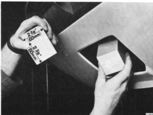
BLOCKS INSERTED BETWEEN HOOD AND RADIATOR FRAME
